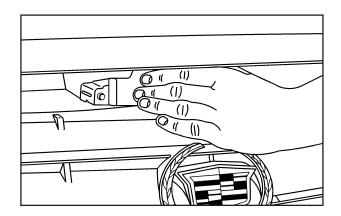
2. Then go to the front of the vehicle and find the secondary hood release lever, located near the center of the hood. Move the release lever up and to the right to raise the hood.
